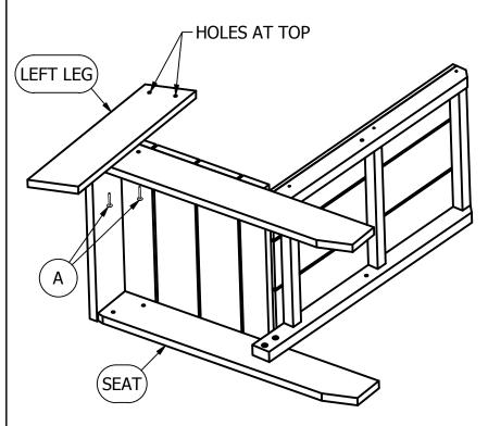
**2)** With Holes Positioned at the Top as Shown, Attach Left Leg to Seat Using (2) "A" Bolts.
